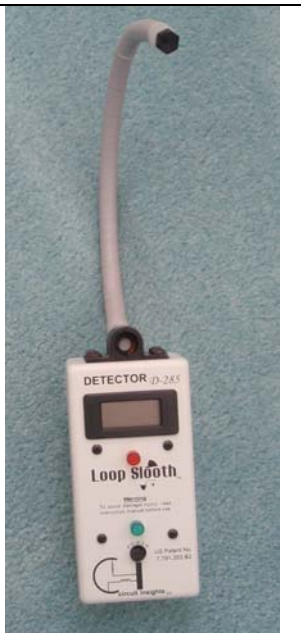
Figure 5. D-285 Detector with Rogowski coil untucked.
